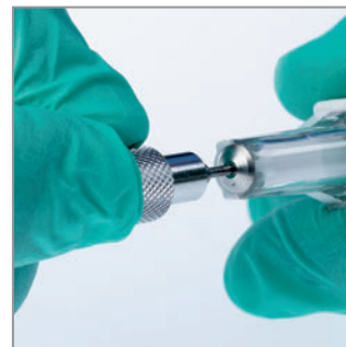
For A New Sharp Edge, Use A 1.25mm Hex Driver Tip To Turn The Blade 90°
